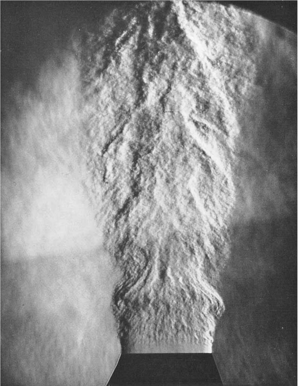
FIGURE 1. Gas-injection schlieren photograph of a 2 in. diameter air jet at a speed of 280 ft/sec (courtesy of Bradshaw et al. 1964). The Reynolds number is 3 \times 10^6 .
